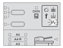
Additionally, the paper jam position lamp blinks to show you where the paper jam has occurred. Check the position and release the jammed paper.
